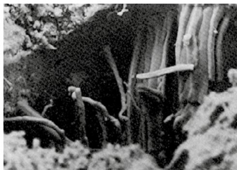
The crystallization of the salts in the pores of the KÖSTER Restoration Plaster prevents the salts from causing damage.
